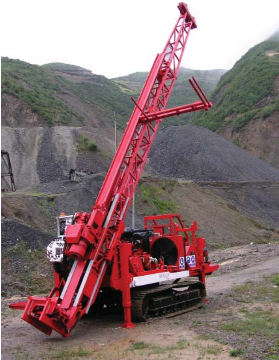
The Diamond Core Drill - DE710 - is used for surface exploration. It's a track mounted drill rig.
